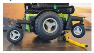
• Place Jack under the front bogie arm pivot
