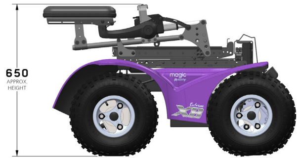
Figure 4.3d Extreme X8 Fold Forward height
