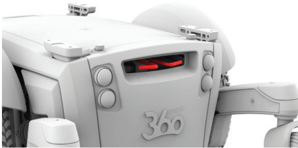
Figure 4.4a Magic 360 brake levers engaged
