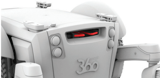
Figure 4.4a Magic 360 brake levers engaged
