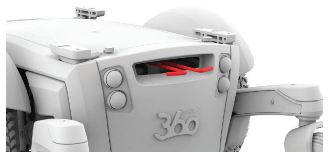
Figure 4.4b Magic 360 brake levers released
