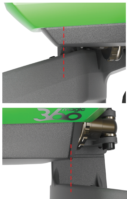
Figure 4.8 - Shock absorber adjustment
