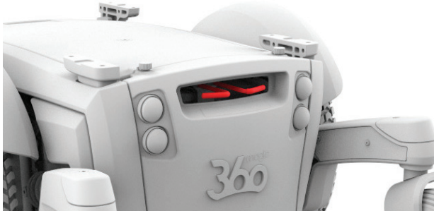
Figure 4.4a Magic 360 brake levers engaged
